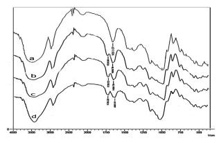
Figure 1. FTIR spectra of native arenga starch (a) and acetylated arenga starches at different of DS: 0.066 (b), 0.208 (c) and 0.249 (d)
