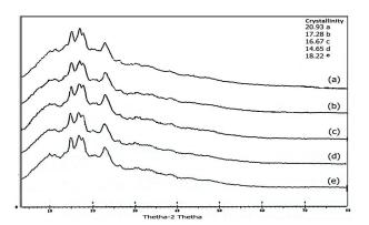
Figure 2. X-ray diffractograms and cristallinity of native arenga starch (a), and acetylated arenga starches with different DS: 0.066 (b), 0.091 (c), 0.208 (d) and 0.249 (e)
